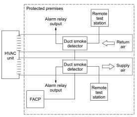
*SuperDuct* detectors continually sample air flow in the HVAC duct and initiate an alarm condition whenever smoke is detected. An alarm is activated when the quantity (percent obscuration) of combustion products in that air sample exceeds the detector's sensitivity setting.
