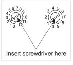
*Example:* for device address 21, set TENS rotary switch to 2 and set the ONES rotary switch to 1.
